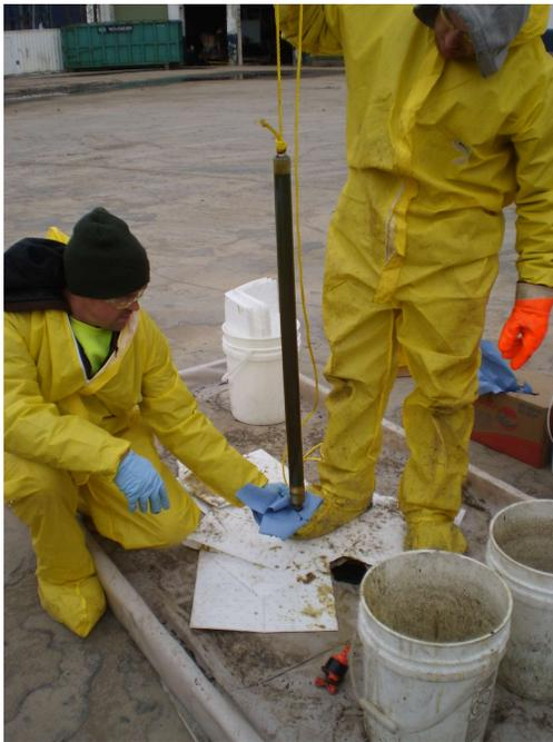
Collected oil and water is poured into buckets prior to containerizing
