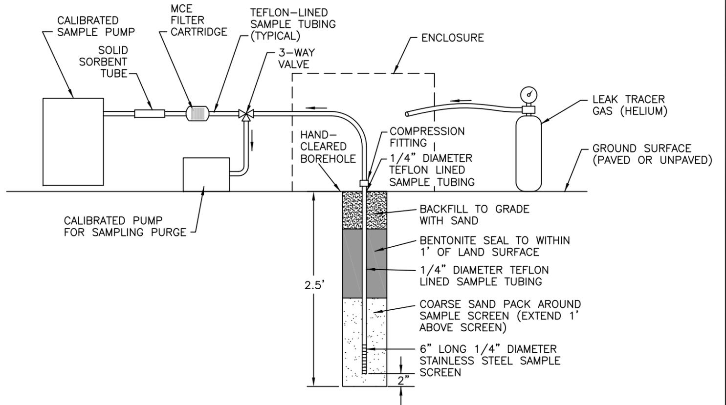
**TYPICAL TEMPORARY SOIL VAPOR MONITORING POINT FOR MERCURY**
