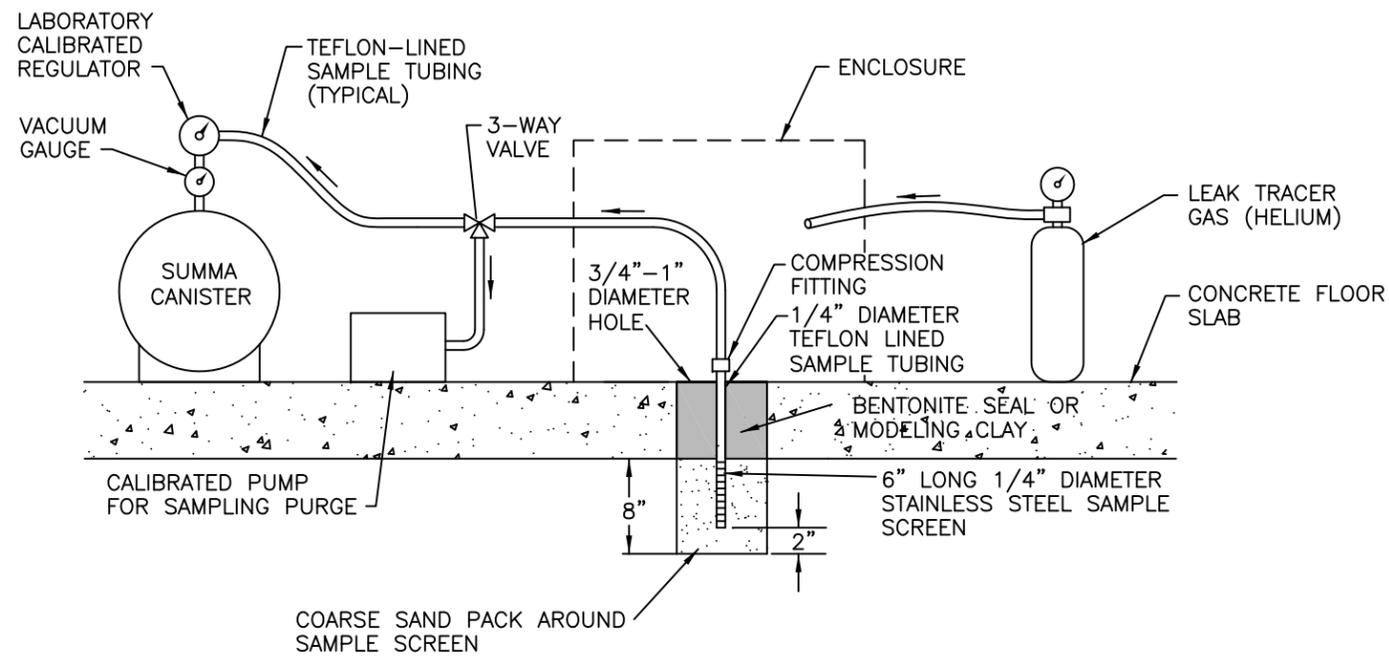
**TYPICAL TEMPORARY SUB-SLAB VAPOR
