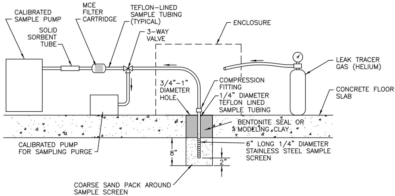
**TYPICAL TEMPORARY SUB-SLAB VAPOR MONITORING POINT FOR MERCURY**
