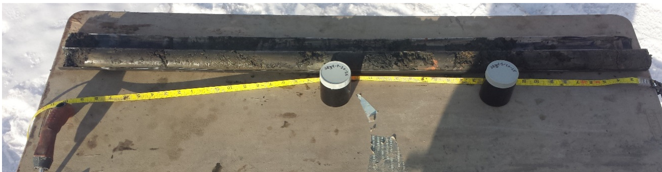
Photo 3: Soil Boring SB34 showing Primary and Secondary sample locations. For the 4 ft cores, depth increases from right to left. Labeled sample jars are shown at the interval where the sample was obtained. (Photo date Jan 16, 2019)
