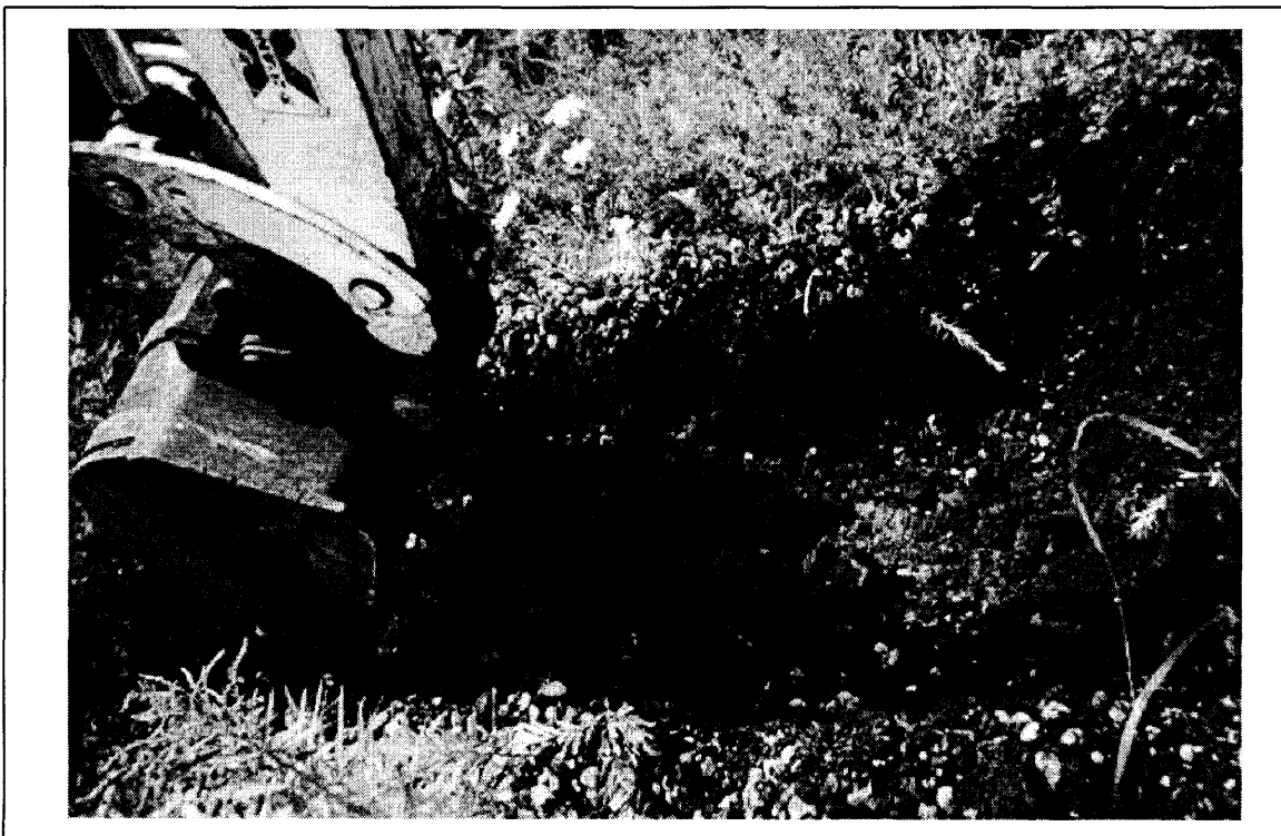
View of TP-03, showing material at 1 fbgs. The red material appears to be paint. No petroleum impacts noted.
