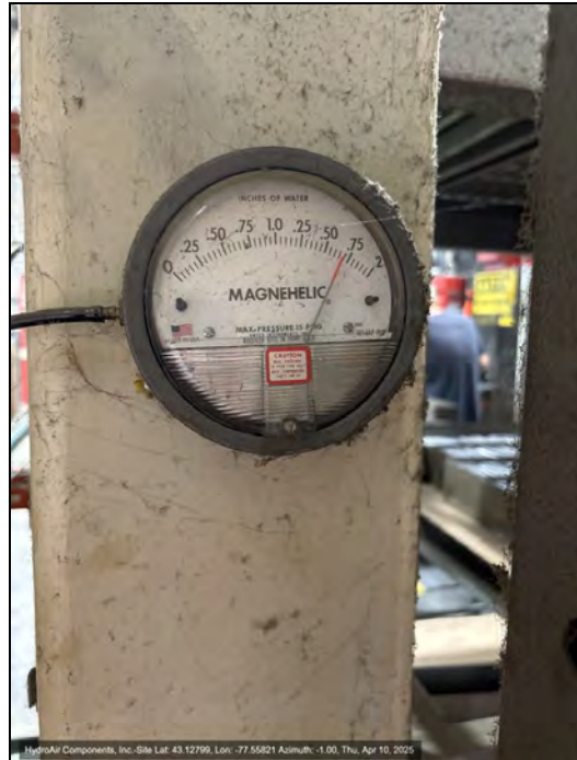
Photo 18: "NW" Magnehelic gauge.
