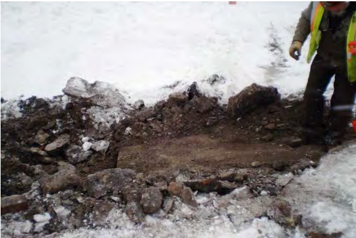
Test Pit 3, concrete slab at north west corner of pit, approximately 8" thick
