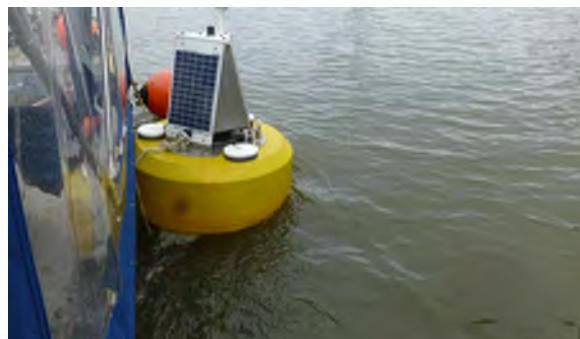
5 Repositioning turbidity monitoring buoys for dredging in DMU's 18 and 19.
