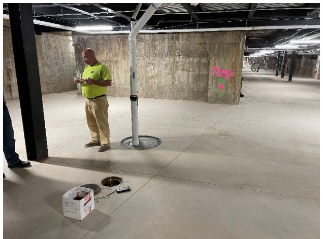
Photo 1: Test Port #1 showing measured pressure differential.
