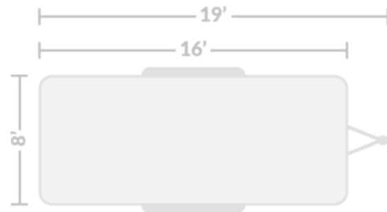
Overhead view of injection trailer dimensions
