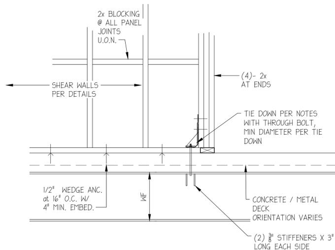
**TYP. SHEAR WALL ON CONC. DECK**
