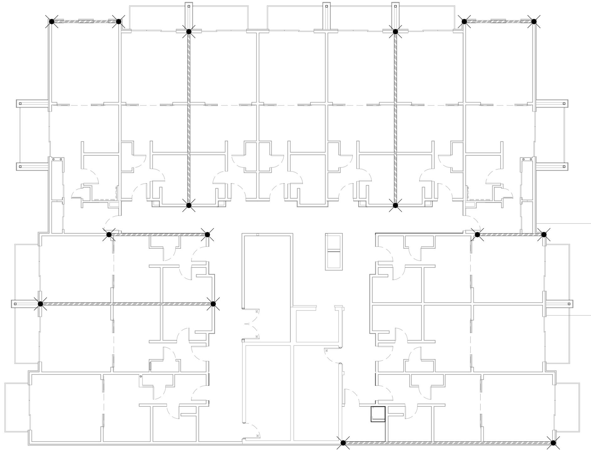
SECOND FLOOR SHEAR WALL PLAN
