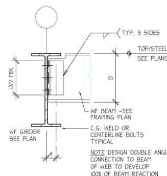
**TYP. FRAMED BEAM CONNECTION DETAIL**
