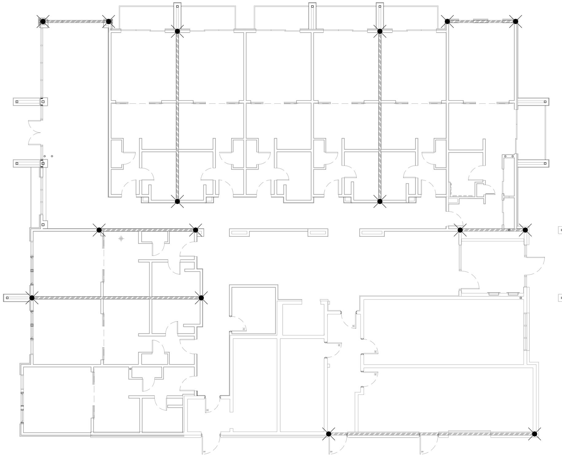
**FIRST FLOOR SHEAR WALL PLAN**
