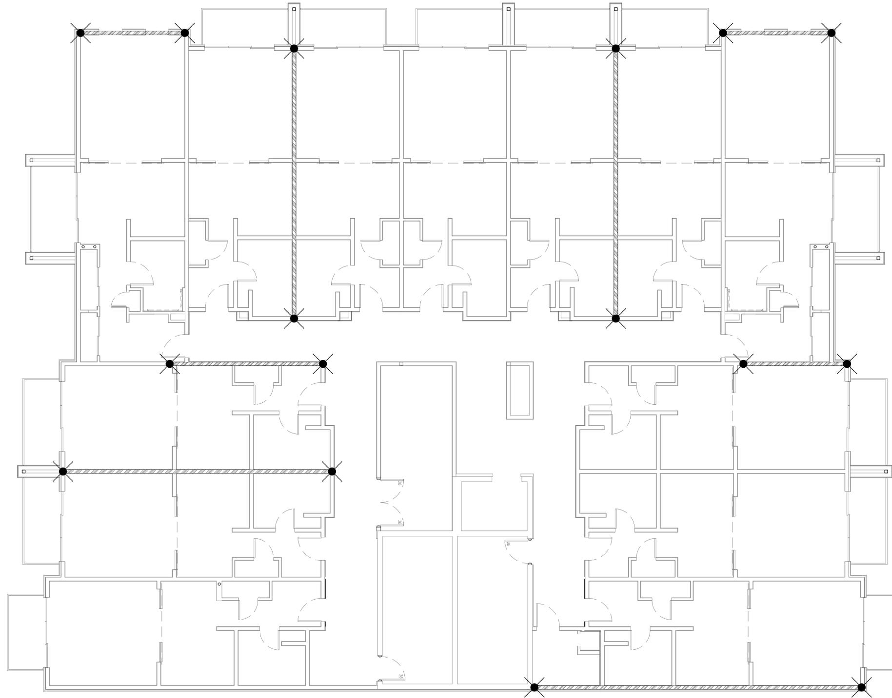
THIRD FLOOR SHEAR WALL PLAN
