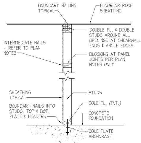
**TYP. SHEAR WALL SECTION**
