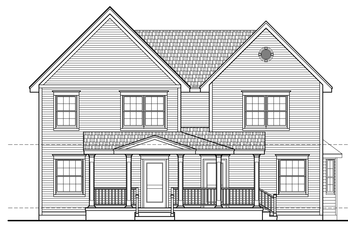
4/3 DOUBLE UNIT (2,803 sq-ft) 4 Bedroom Unit (1,521 sq-ft) 3 Bedroom Unit (1,281 sq-ft) FRONT ELEVATION SCALE 1/8" = 1'-0"
