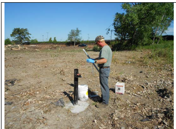
11. Between 10 to 15 well volumes are bailed out of each well
