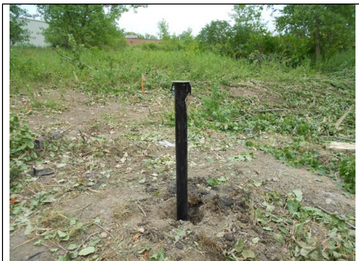
16. The protective casing that covers the riser at MW-6
