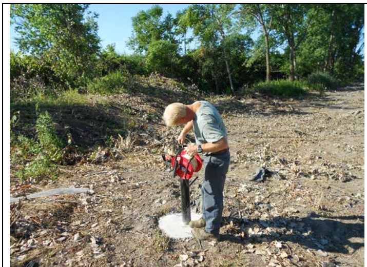
10. The depths of each MW are measured during development
