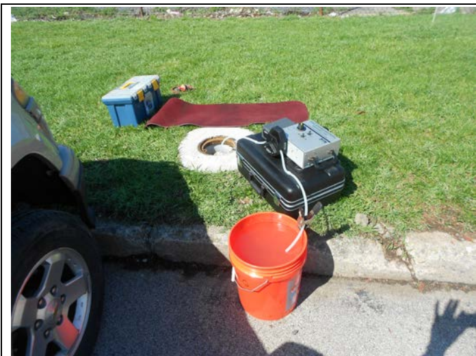
1. Low flow sampling set up at MW-3
