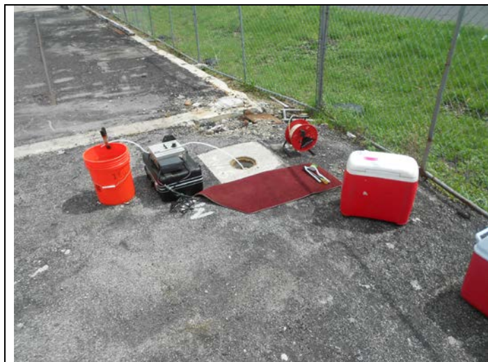
3. Low flow sampling set up at MW-4
