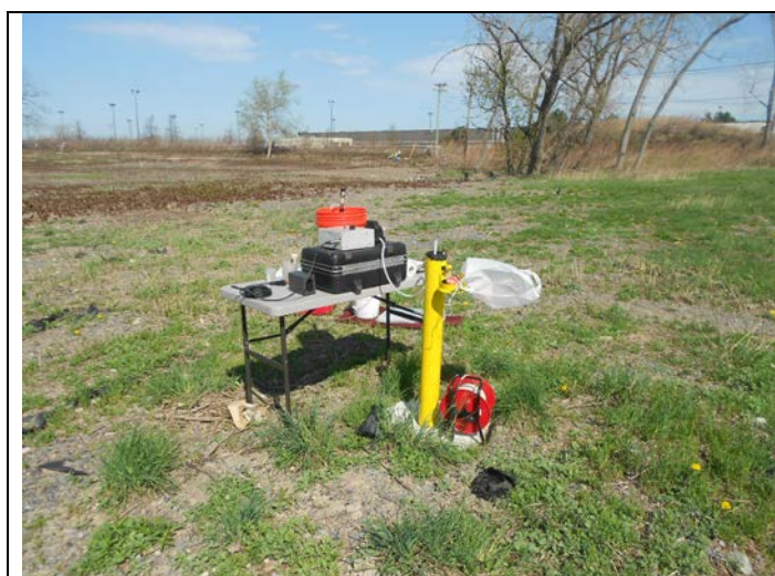
5. Low flow sampling set up at MW-7
