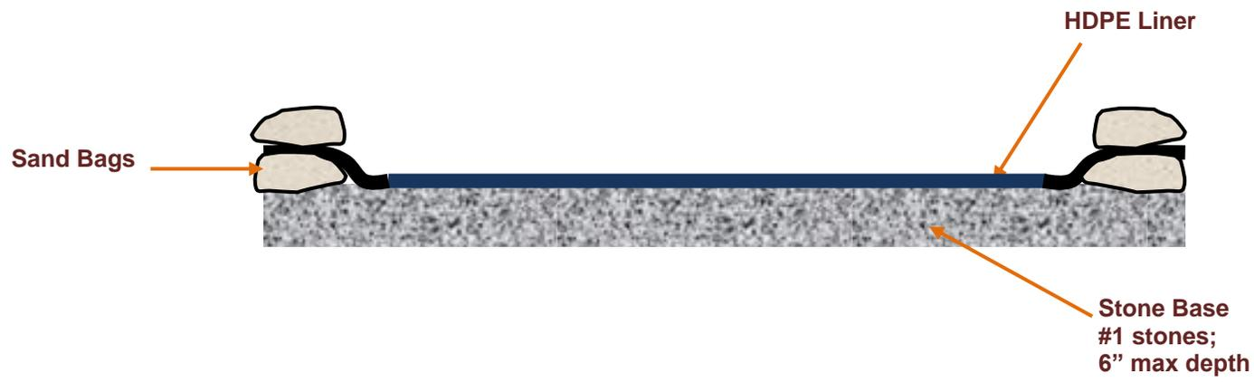
Note: Decon pad is sloped to one corner with sump to collect wash water for treatment
