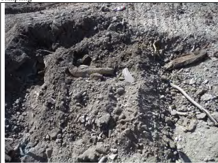
3. Close view of a GS-17 test pit used for composite sampling
