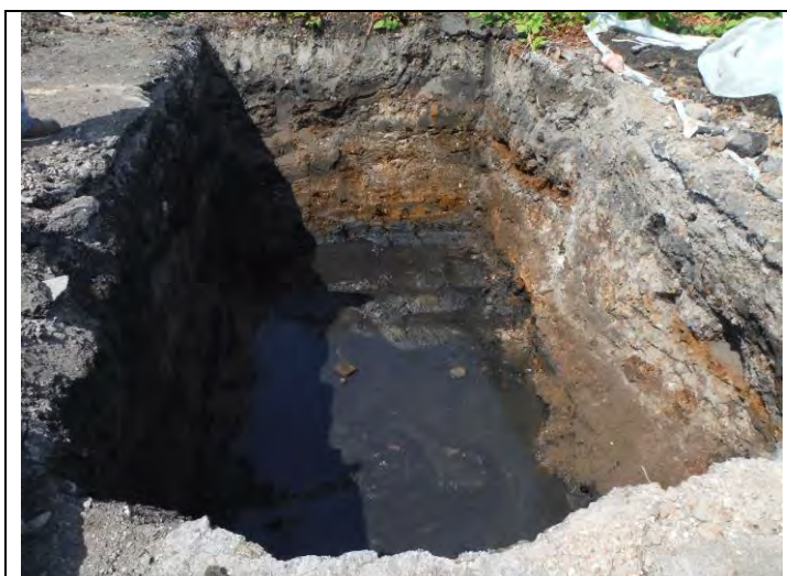
6. MW-2 contained very dark material below 4' and had a slight sheen on the ground water
