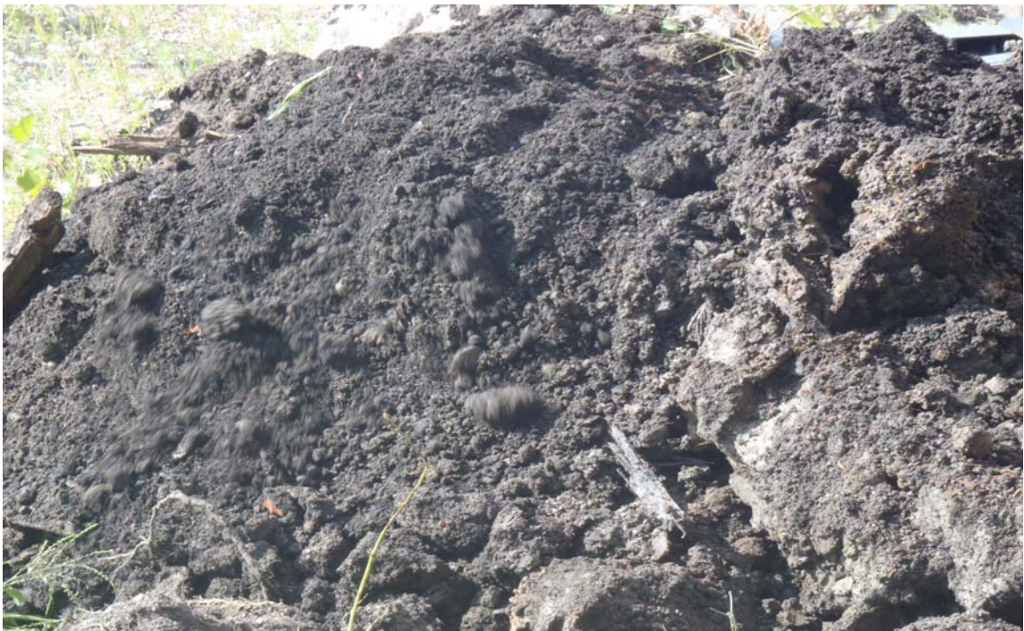
Photograph 6 –Test Pit TP-3 – Typical Fill Removed from Test Pit
