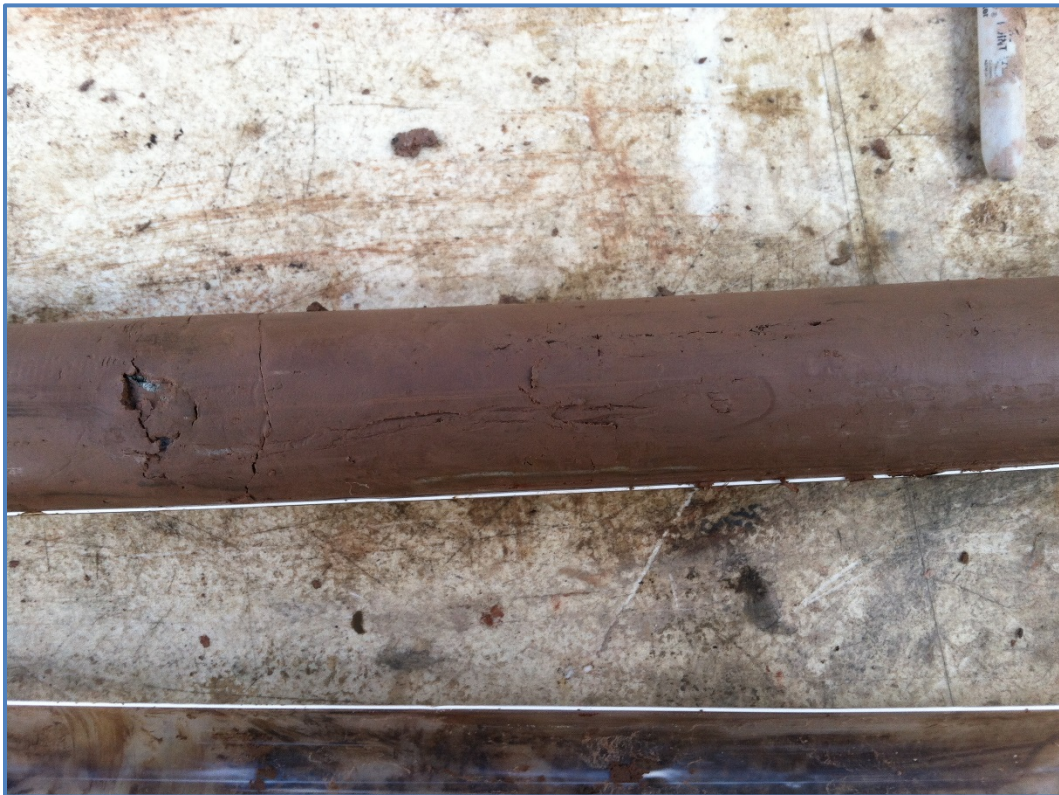
Figure 5-6. Close-up photo of the native reddish brown silty clay from soil boring SB-37 at the Highland Plaza Off-Site Area. Photo taken by Glenn M. May on May 4, 2017.
