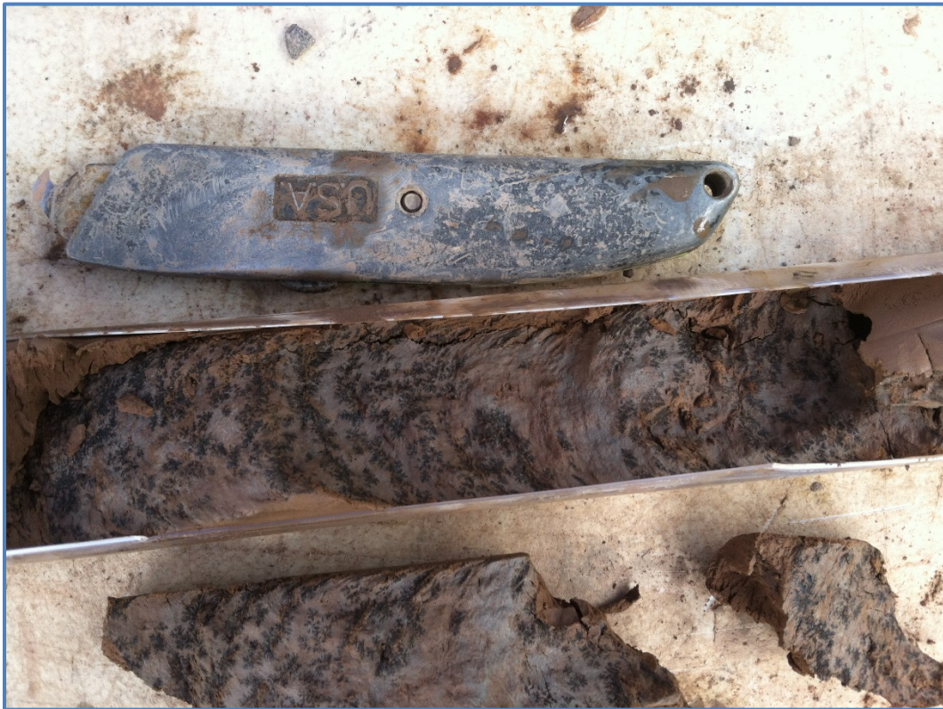
Figure 5-7. Close-up photo showing mottling of the native reddish brown silty clay in soil boring SB-52 at the Highland Plaza Off-Site Area. Photo taken by Glenn M. May on June 22, 2017.
