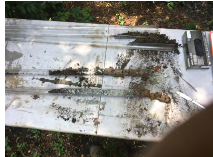
20. BH-1 soil core. 0 – 8', top to bottom, left to right.
