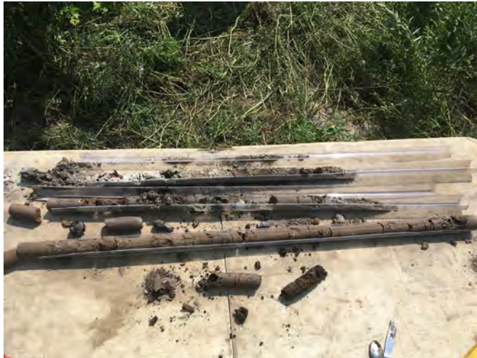
3. BH-1 soil core. 0 -12' top to bottom, left to right.
