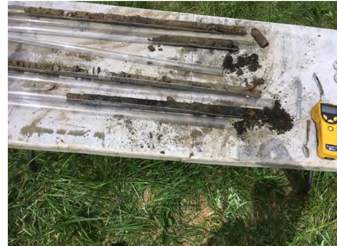
24. BH-6 soil cores. 0 – 6' top to bottom, left to right.
