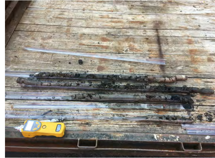
14. BH-4 soil core. 0 – 12' top to bottom, left to right.
