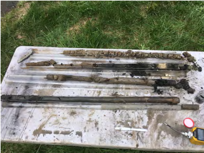
23. BH-5 soil core. 0 -16' top to bottom, left to right.
