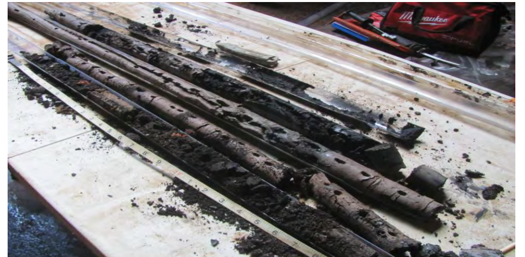
4. Borehole SBH-1 soil cores
