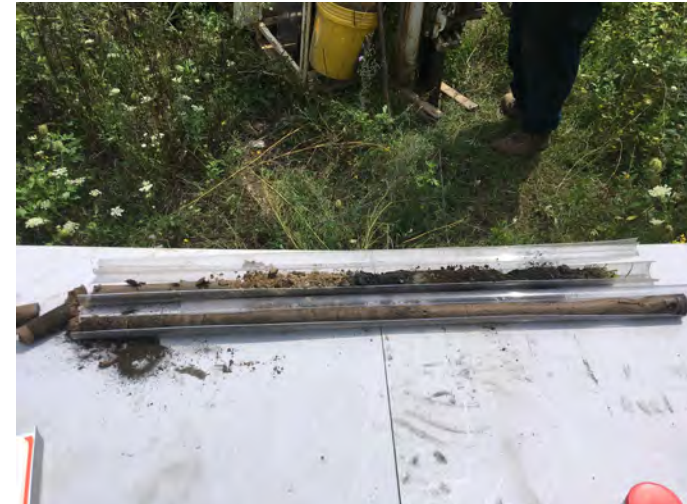
8. BH-4 soil core, 0 – 8' top to bottom, right to left.
