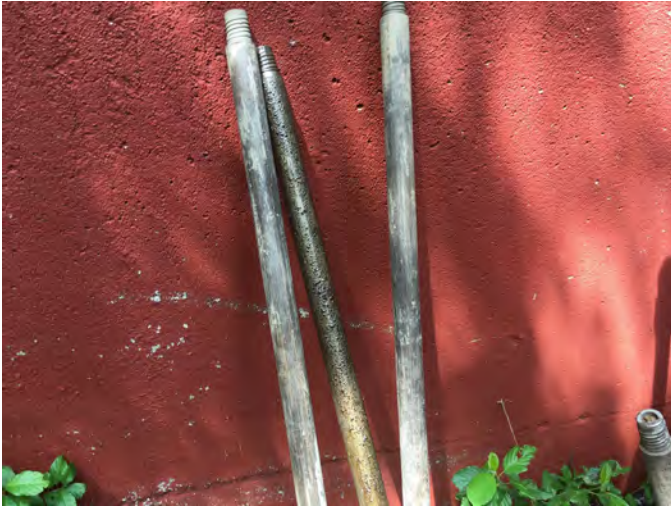
21. Product found on probe rods after BH-1 boring.
