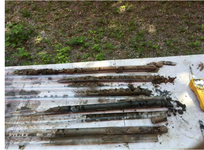
18. BH-2 soil core. 0 – 16' top to bottom, left to right.
