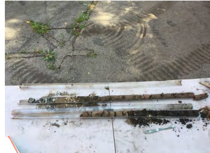
16. BH-3 soil core. 0 – 6' top to bottom, left to right.
