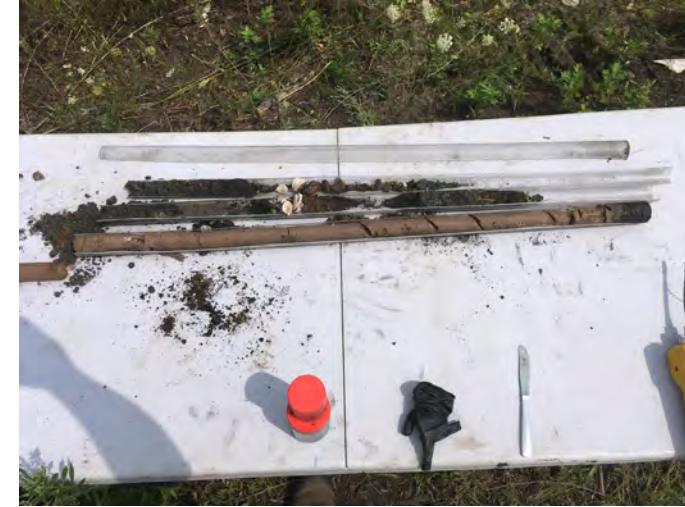
10. BH-5 soil core. 0 – 8'; top to bottom, right to left.
