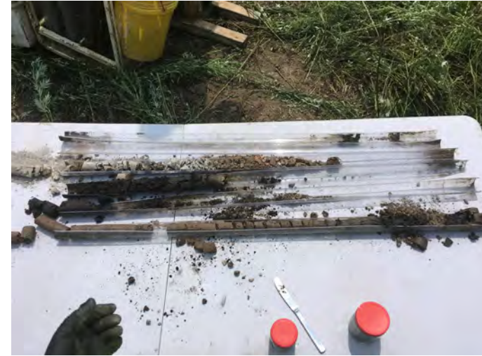
6. BH-3 soil core, 0 – 11' top to bottom, right to left.
