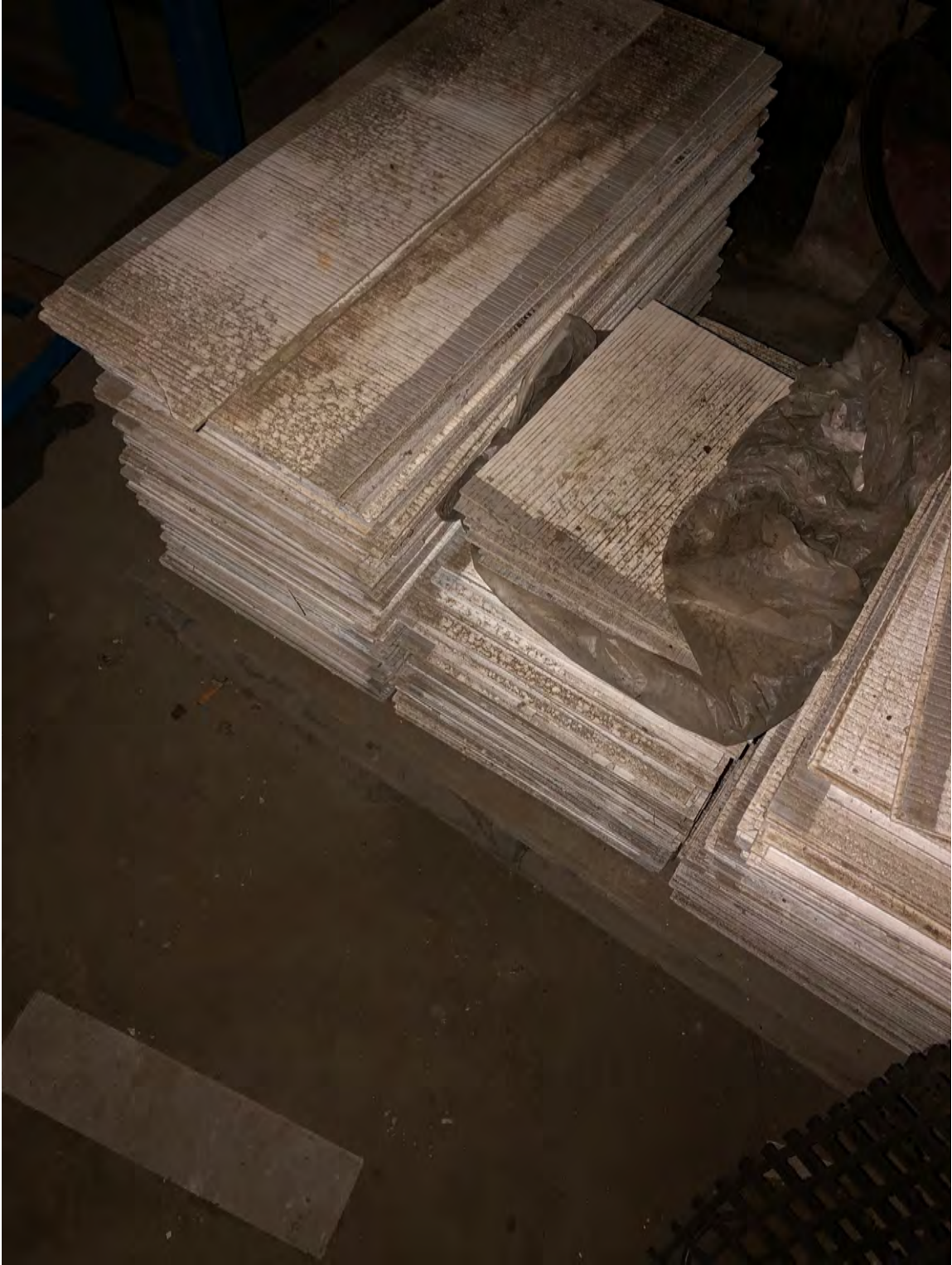
Transite Siding Stacked on a Pallet
