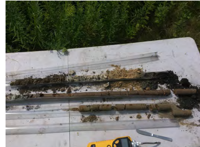
12. BH-6 Soil core. 0 – 9' top to bottom, left to right.
