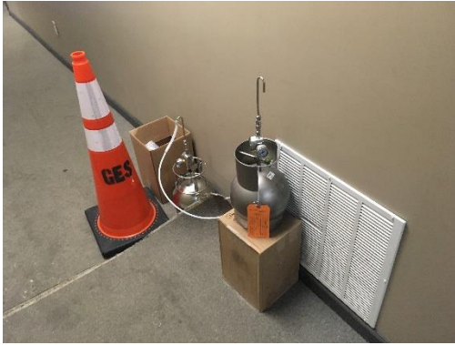
Image 6: Summa Canisters Sample Location: Main Hallway
