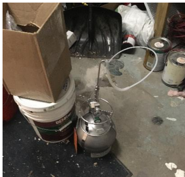
Image 16: Sub-slab Canister Sample Location: Garage 1
