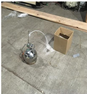
Image 10: Sub-slab Canister Sample Location: Room #5
