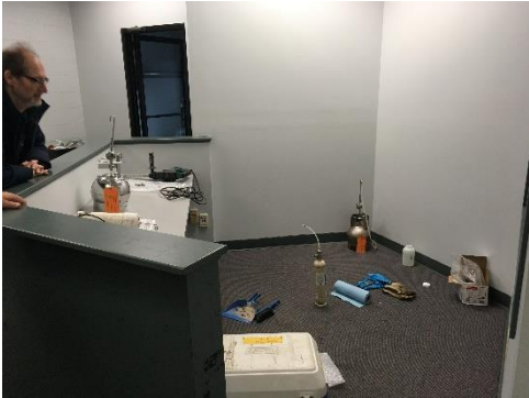
Image 8: Indoor Air Summa Canister Sample Location: Front Lobby (On Desk)
