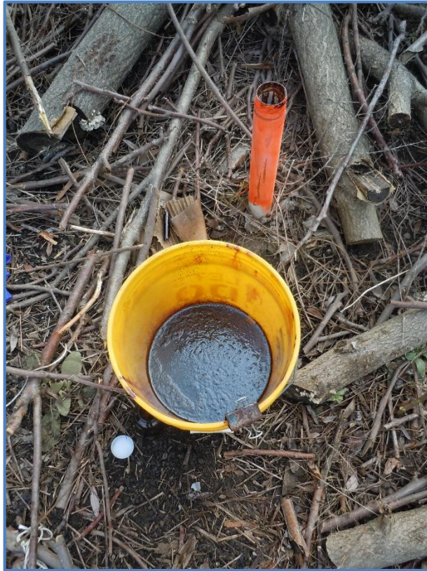
Figure 4-1. Photo showing the NAPL extracted from monitoring well 1660-MW-7 during sample collection. Photo taken by Glenn M. May on January 15, 2020.
