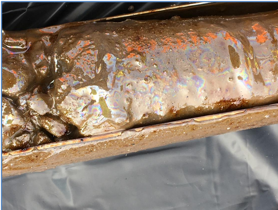
Figure 4-6. Photo showing NAPL and sheens in the gravelly sand deposit in soil boring 1660-MW-5R. Photo taken by Glenn M. May on September 14, 2020.
