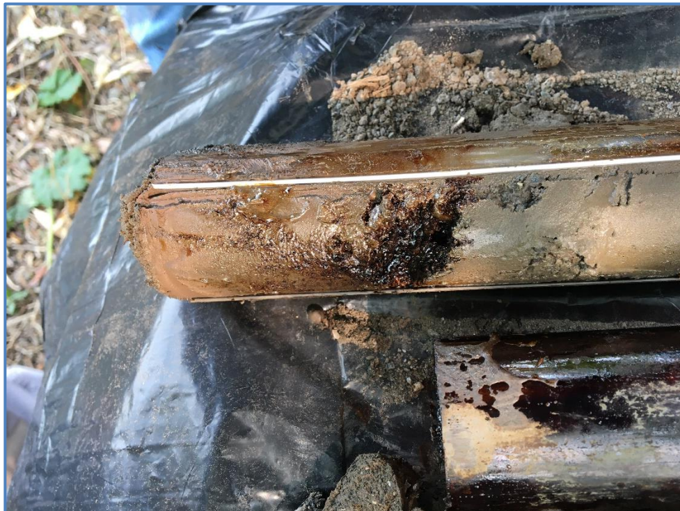
Figure 4-8. Photo showing NAPL in a sand seam in soil boring 1660-MW-8. The underlying reddish-brown silty clay is also shown. Photo taken by Glenn M. May on September 16, 2020.
