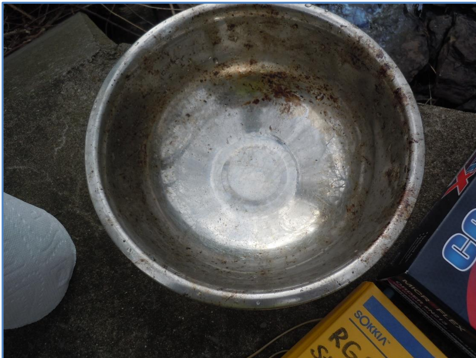
Figure 4-4. Photo showing the viscous, brownish black, sticky residue in the sampling bowl following the collection of sediment sample SED-1. Photo taken by Glenn M. May on January 15, 2020.
