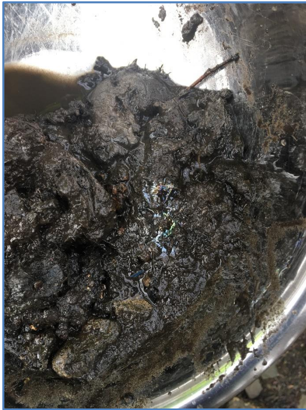
Figure 4-5. Photo showing the rainbow sheen on sediment sample SED-2. Photo taken by Glenn M. May on January 15, 2020.
