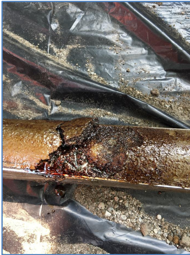
Figure 4-7. Photo showing NAPL in a sand seam in soil boring 1660-SB-1. Photo taken by Glenn M. May on September 16, 2020.
