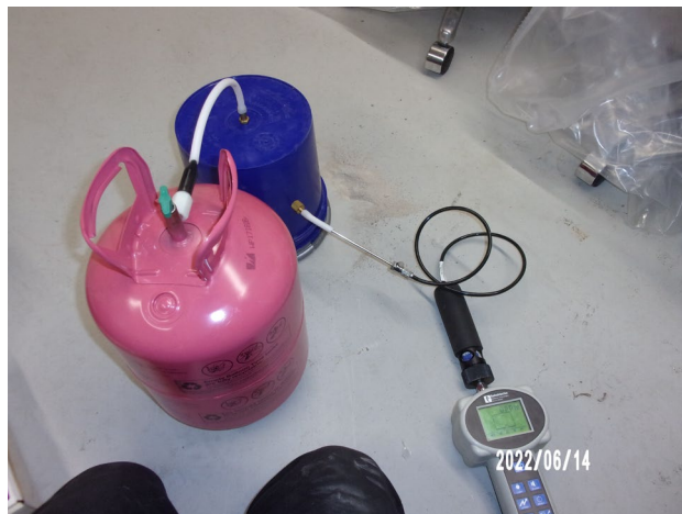
6. Helium tracer test performed at SS-12(061422) in the basement storage area.
