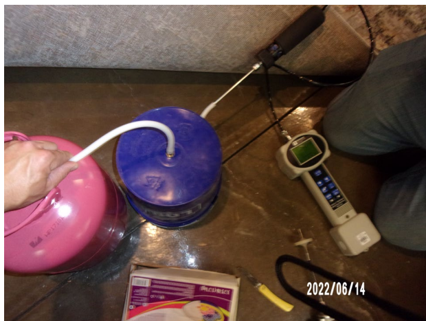
3. Helium tracer test performed at SS-13(061422) in the ODL waiting room.
