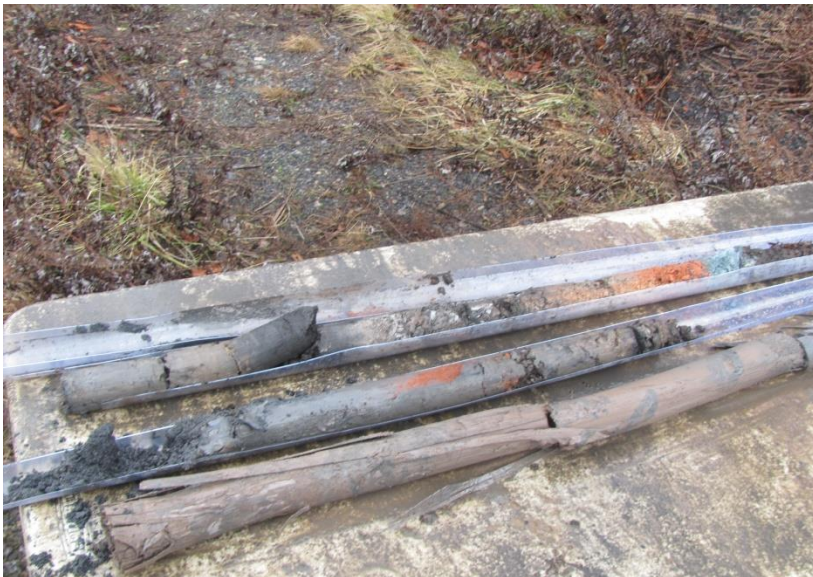
59. Soil cores from BH-9A - 2017
