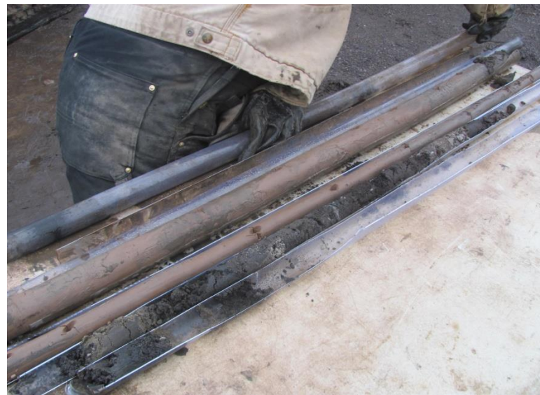
34. Soil cores from BH-1A - 2017
