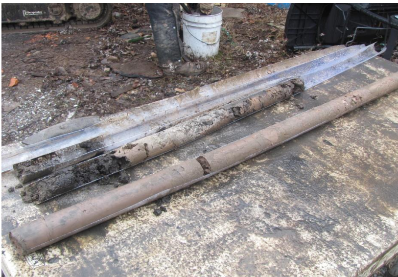
53. Soil cores from BH-7A - 2017
