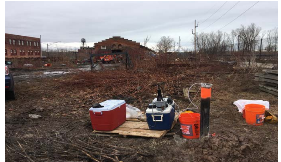
76. MW-1 location and low flow pump sampling set up, facing south
