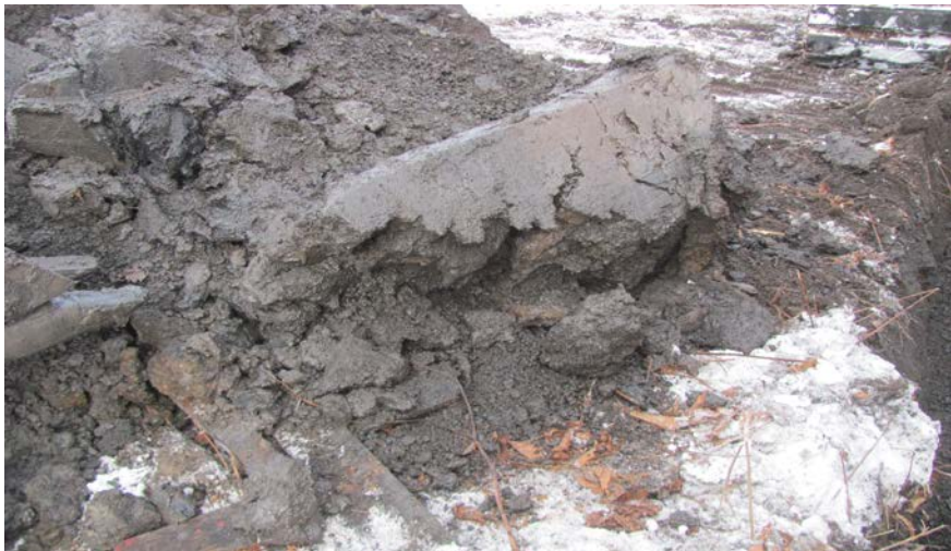
51. View of excavated clay-gravel interface material from TP-6
