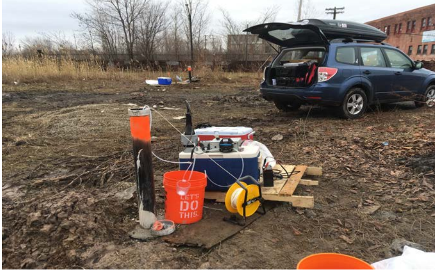
77. MW-1 location and low flow pump sampling set up, facing east
