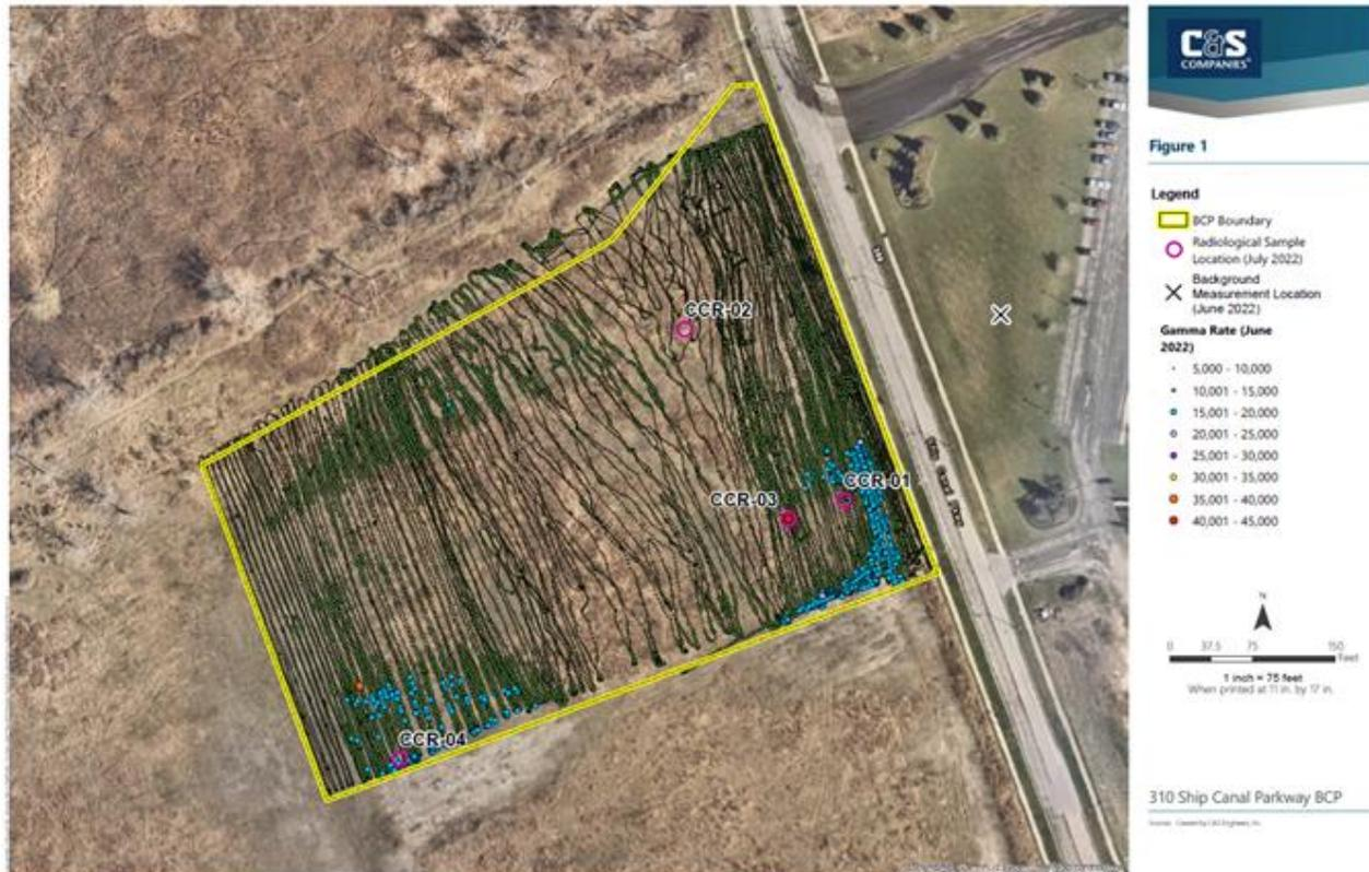
**Figure 1.** 310 Ship Canal Parkway Gamma walkover survey and soil sample locations.
