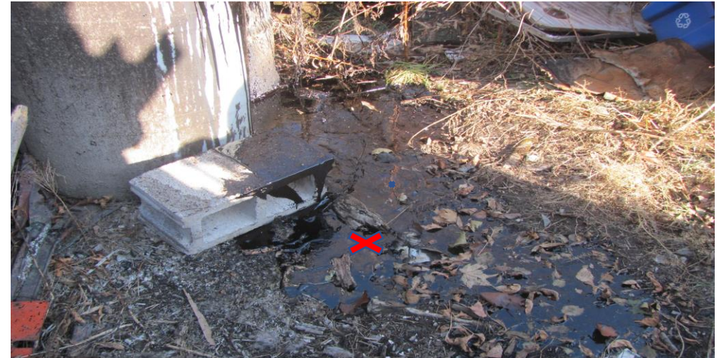
36. Surface soil 3 location adjacent to B9 and leaking drums. Drums reportedly filled with fuel oil tank bottoms
