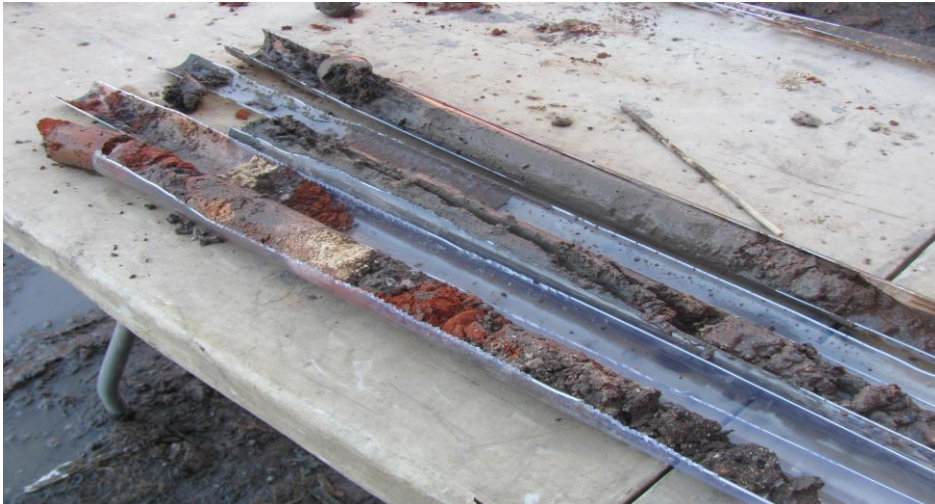
35. Soil cores BH-10. Note supposed location of former fuel oil tank
