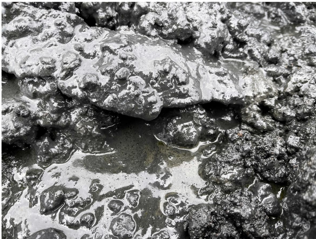
Photograph No. 2: The sample of fill from below the Former Light Oil Building slab had observable black NAPL blebs.
