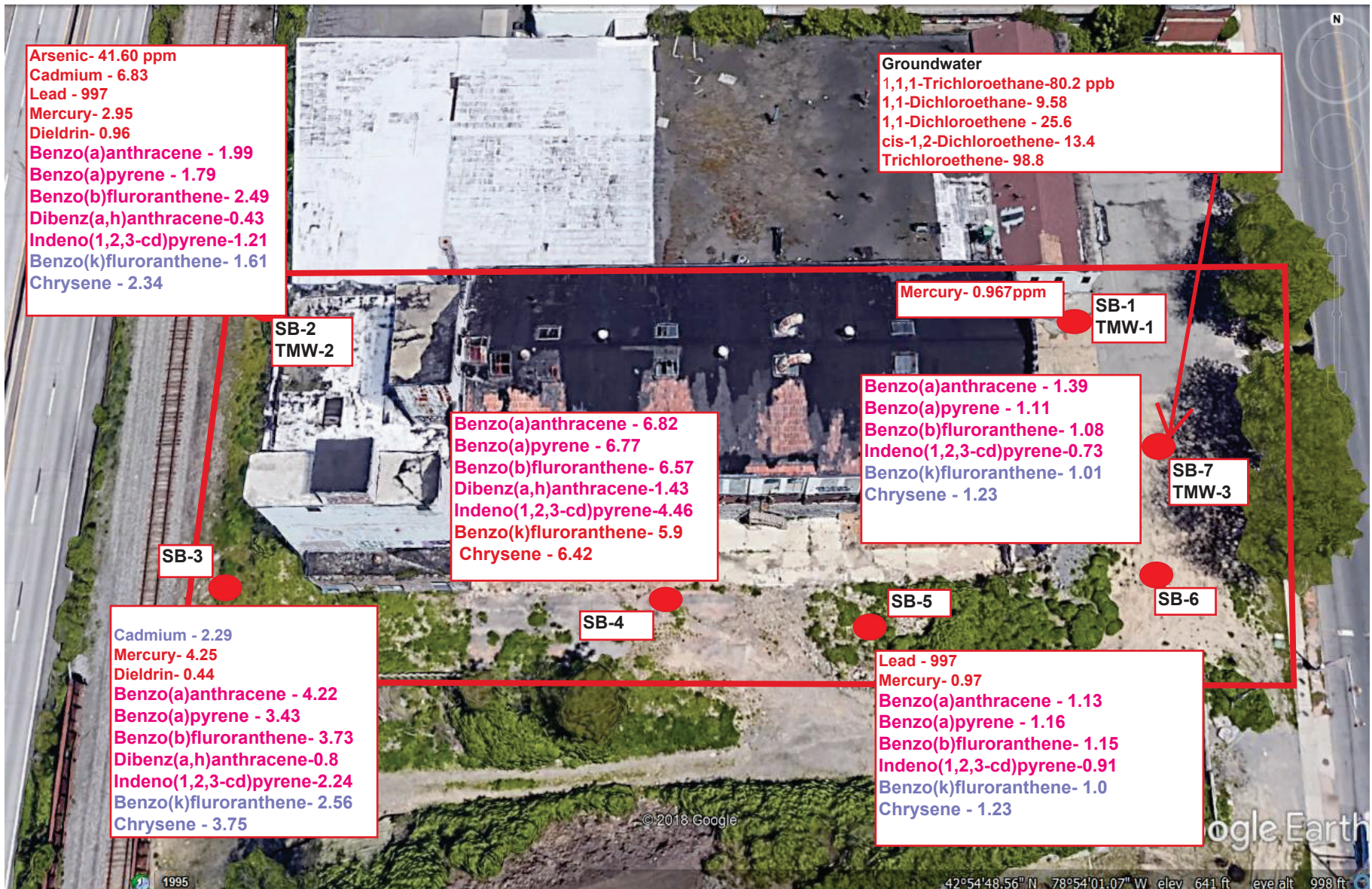
Figure 11: Location of Soil Borings (SB) and Temporary Monitoring Wells with Analytical Results Notes: Red- Greater than restricted residential SCOs or TOGs; Blue - greater than unrestricted & Residential SCOs
