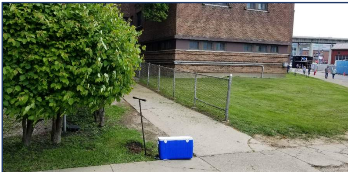
Photo 3 – Hand auger boring at EB-09.
