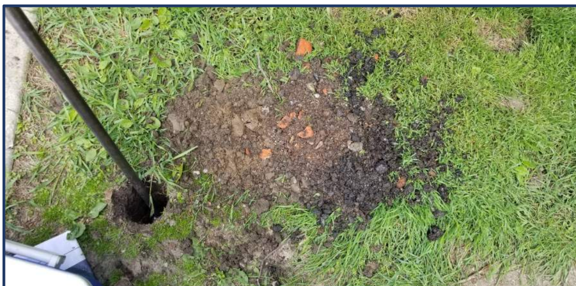
Photo 4 – View of typical urban fill material observed throughout the Site.
