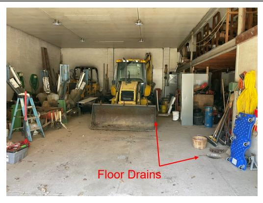
Photograph 11: Inside Building 6, apparently used as a garage and office area for the former nursery. Filled with equipment and materials associated with the former nursery. Two floor drains were identified within the garage, one shown on the right side of this photo (Eastern Floor Drain) and the other located behind the loader bucket (Western Floor Drain) (looking west).
