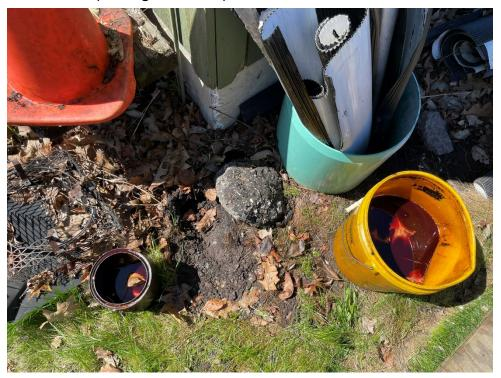
Photograph 10: The 5-gallon bucket was moved aside to sample underlying soil (HA-20). Grossly contaminated material was identified in the soil (black staining, strong petroleum odors, PID reading of 60 ppm).
