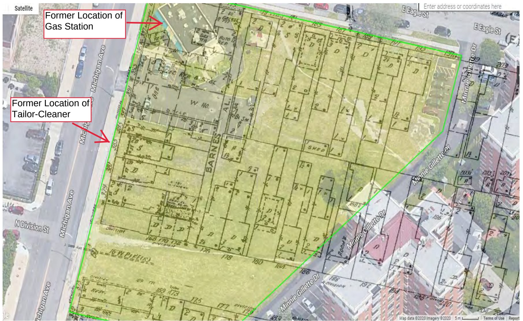
FIGURE 1B: 2017 Aerial with 1950 Sanborn Overlay
