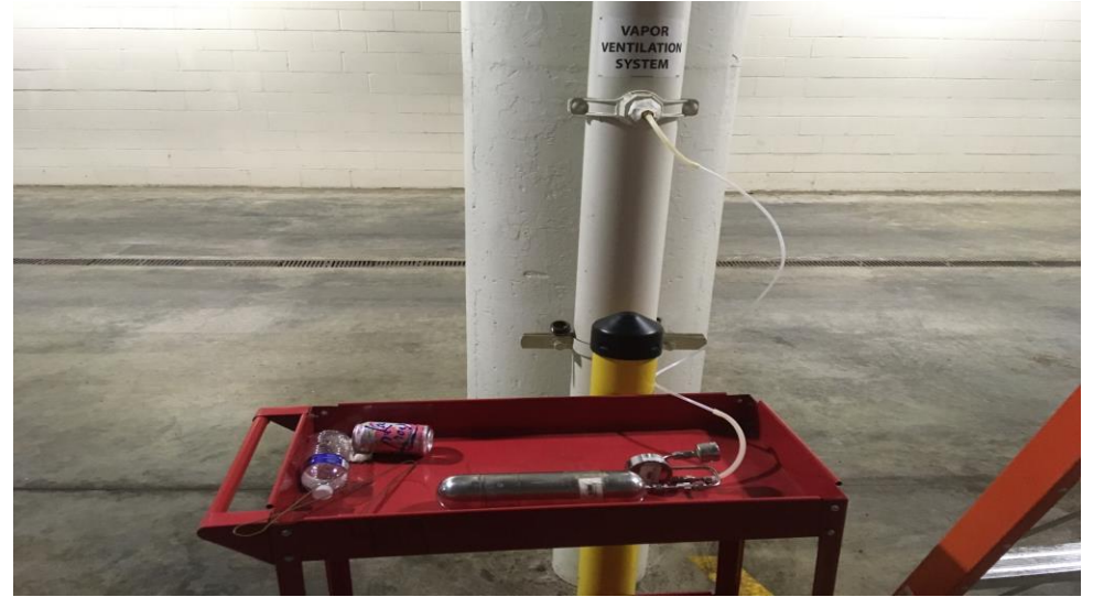
14. Air Sampling of Vapor System
