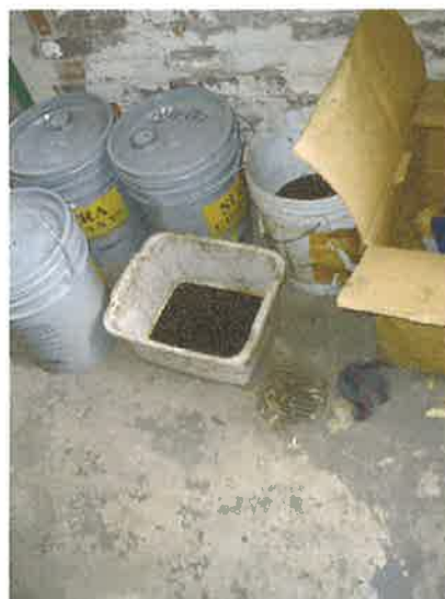
Compressor oil staged in compressor building (Building S). Note floor drain to right of wash tub containing oil.
