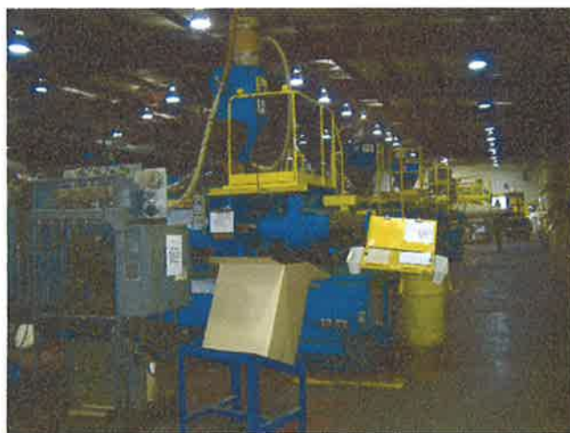
Building Q-1 injection molding equipment for larger parts. Water and hydraulic oil noted on floor, facing north.
