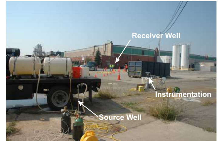
Installation of Hydraulic Pulse Interference Test Equipment
