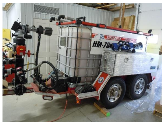
Image 30: "NYS Foam Trailer" outfitted with two 330-gallon totes of National Foam - Universal Gold 1%-3% AR-AFFF foam concentrate.
