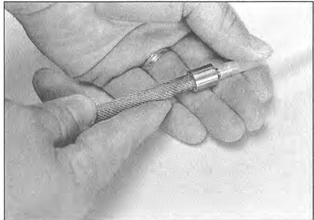
Attaching polyethylene tubing to the sampling implant.
