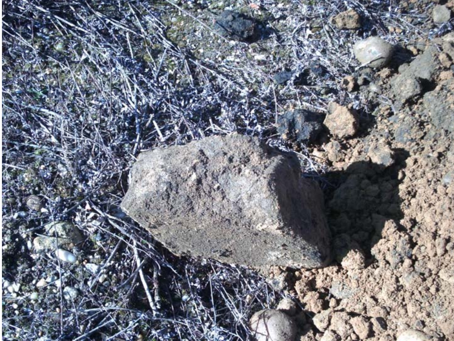
Large piece of concrete found at two feet below grade.
