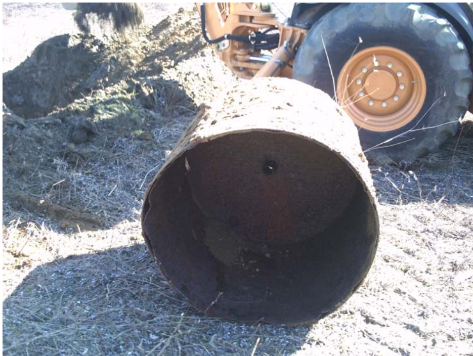
The object was a three foot diameter hollow steel cylinder with a solid end on one side.
