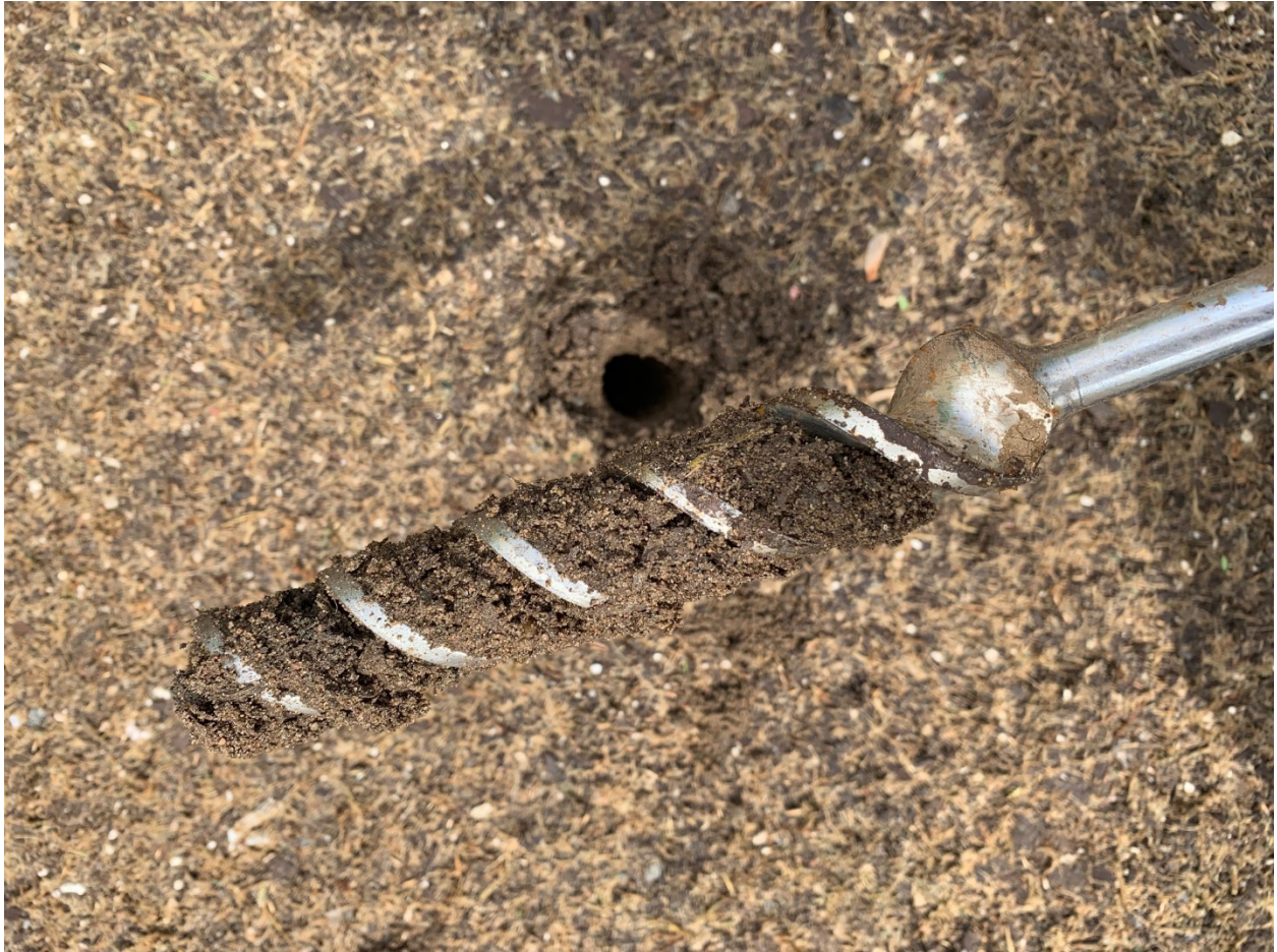
Figure 3 Soil auger of topsoil mix showing a minimum of 6" compacted soil mixture
