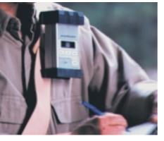
The personalDataRAM's rugged, yet attractive, brushed extruded aluminum case is designed to protect the unit's optics and electronics in even the harshest industrial environments. Heavy-duty molded bumpers shield the monitor from inadvertent mishandling and moderate impact. The absence of any moving parts (e.g. pumps, motors, valves, etc.) and the use of low-power semiconductor components throughout ensures long life and failure-free operation
