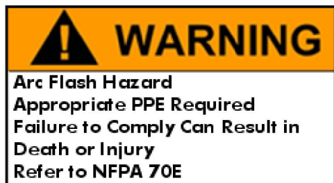
Minimum arc flash label example
