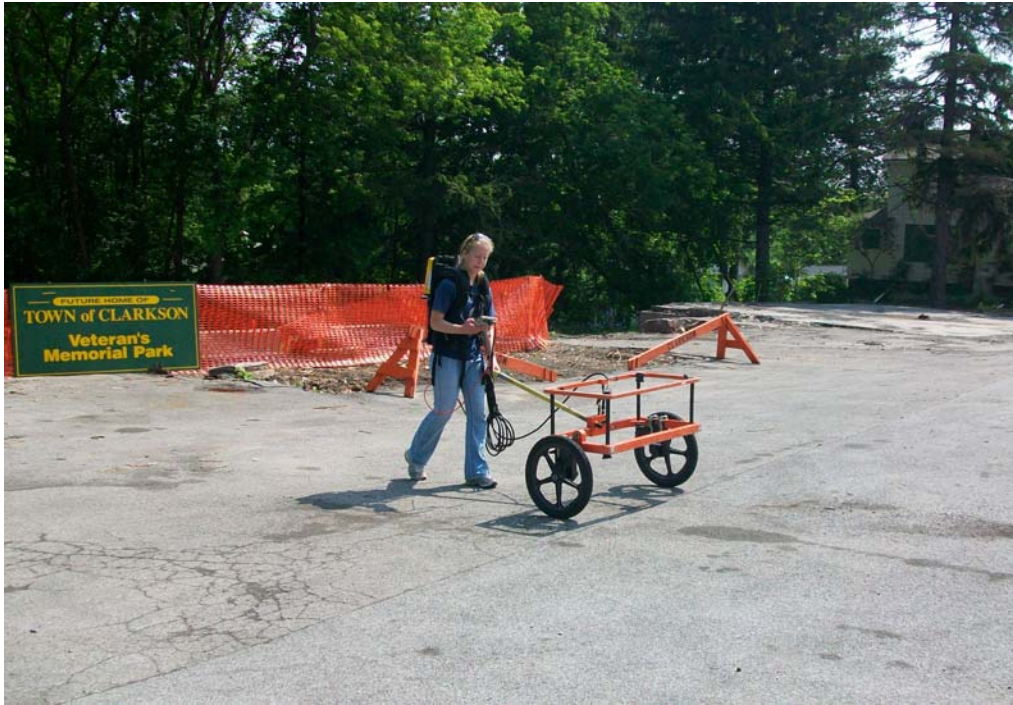
Photo No. 3. EM-61 geophysical survey.
