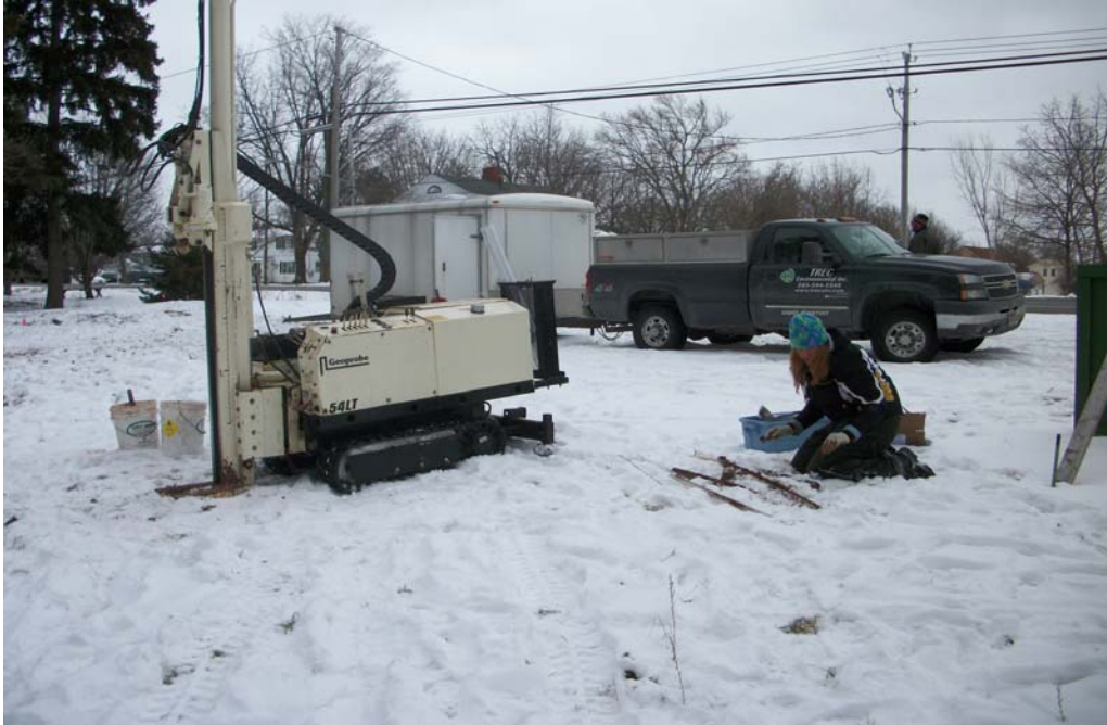
Photo No. 7. View of Geoprobe used for soil borings.
