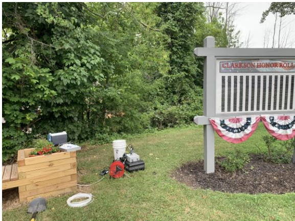
Photo No. 3 Low-flow sampling setup at MW-04
