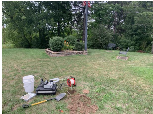
Photo No. 4 Low-flow sampling setup at MW-01
