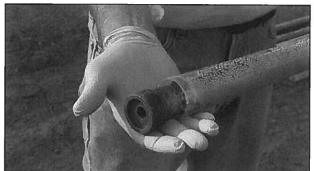
Figure 4.32. MC5 Closed Piston Point is retrieved from the top of the liner.
