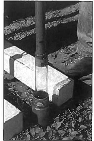
Figure 4.20. Lower liner to bottom of outer casing on leading end of inner rods.
