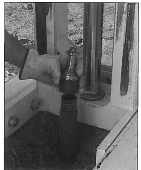
Figure 4.26. The pull cap is one way to remove the sampler from the ground.
