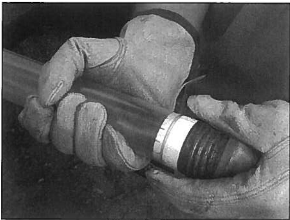
Figure 4.18. Place either end of the liner onto the spacer ring or core catcher. The liner should fit securely.
