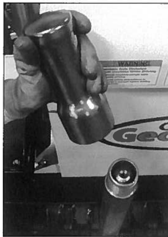
Figure 4.22. Place a DT22 Drive Cushion Assembly on top of the inner rods and a drive cap onto the outer casing.
