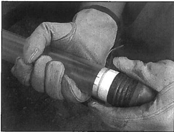
Figure 4.6. Place either end of the liner onto the spacer ring or core catcher. The liner should fit securely.
