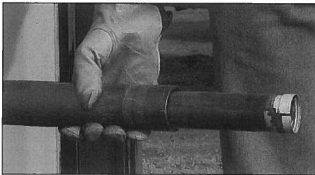
Figure 4.29. Remove the MC5 Cutting Shoe and liner from the MC5 Sampler Tube.
