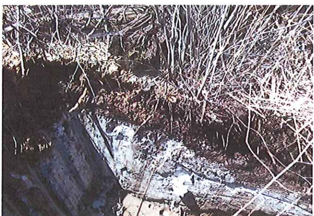
Photograph 15. Lime material within PEI-TP-15
