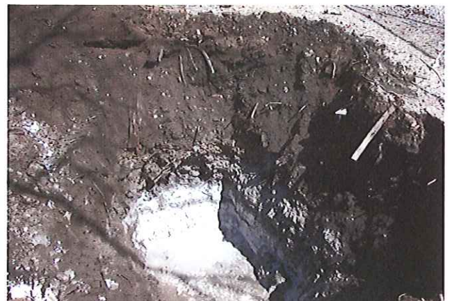
Photograph 4. Lime and groundwater within PEI-TP-02
