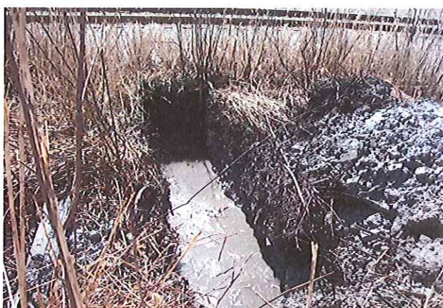
Photograph 16. Groundwater within PEI-TP-16
