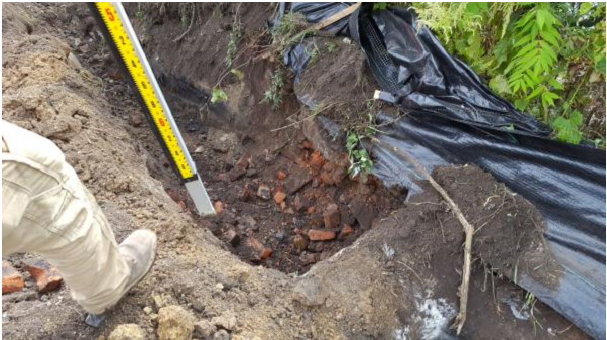
Photo 3 : Fills (predominantly C&D debris) encountered at southwestern corner of drain alignment.
