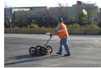
Malå RAMAC/Ground Penetrating Radar (GPR) system with a 250 MHz antenna
