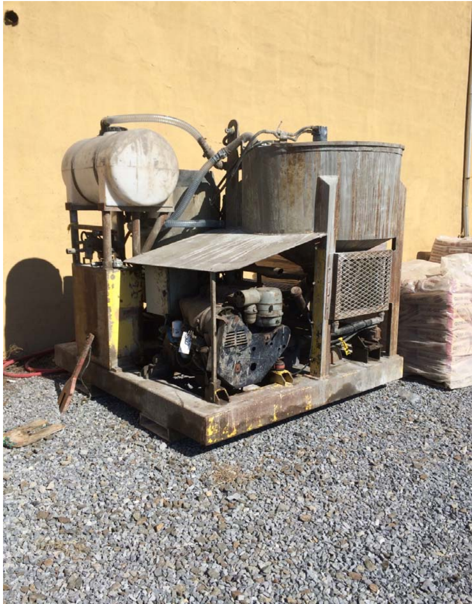
Photo 3: High shear grout mixer onsite, March 1, 2016
