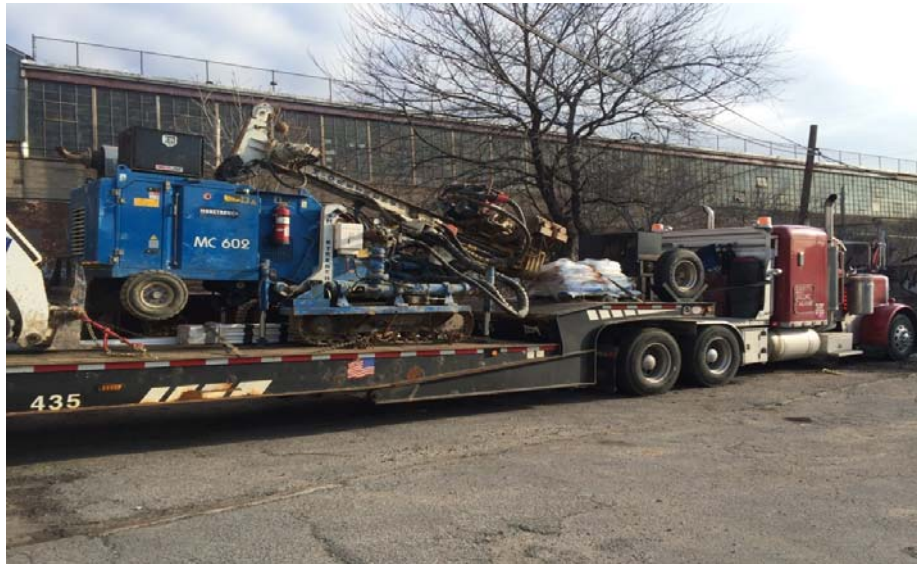
Photo 1: Mobilization of Comacchio drill rig, March 1, 2016
