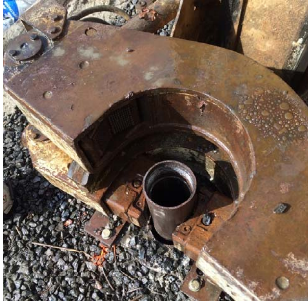
Photo 8: Drill rig with 5.5 inch drill casing, March 3, 2016
