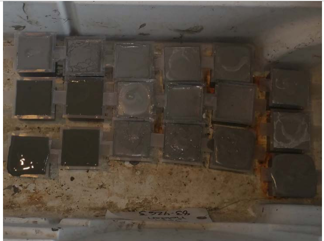
3/10/16- Grout sampled by contractor- 2 inchx2inch grout cubes.
