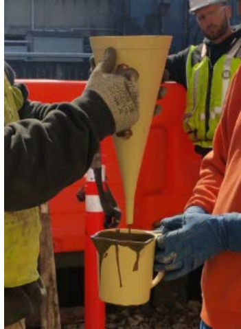
3/08/16 - Grout consistency checked with marsh funnel.
