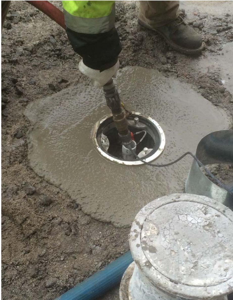
Photo 17: Slug Test being performed at PZ-4, March 14, 2016
