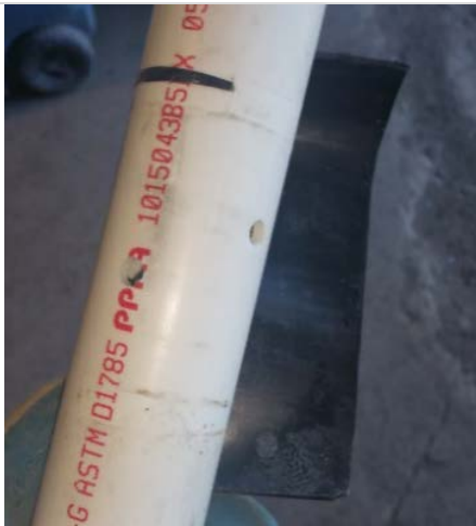
3/02/16- 1 1/2" dia PVC pipe with 1/4" dia. Drilled hole.
