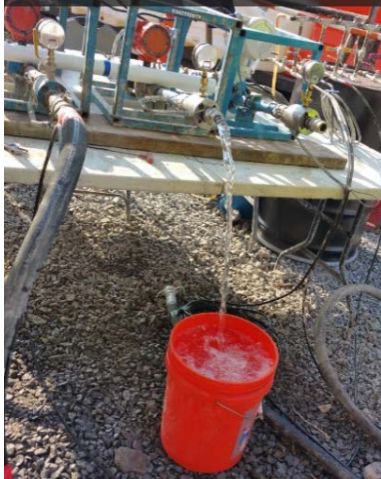
3/07/16 - Flowmeter calibration was checked by passing volume of water through the flowmeters.
