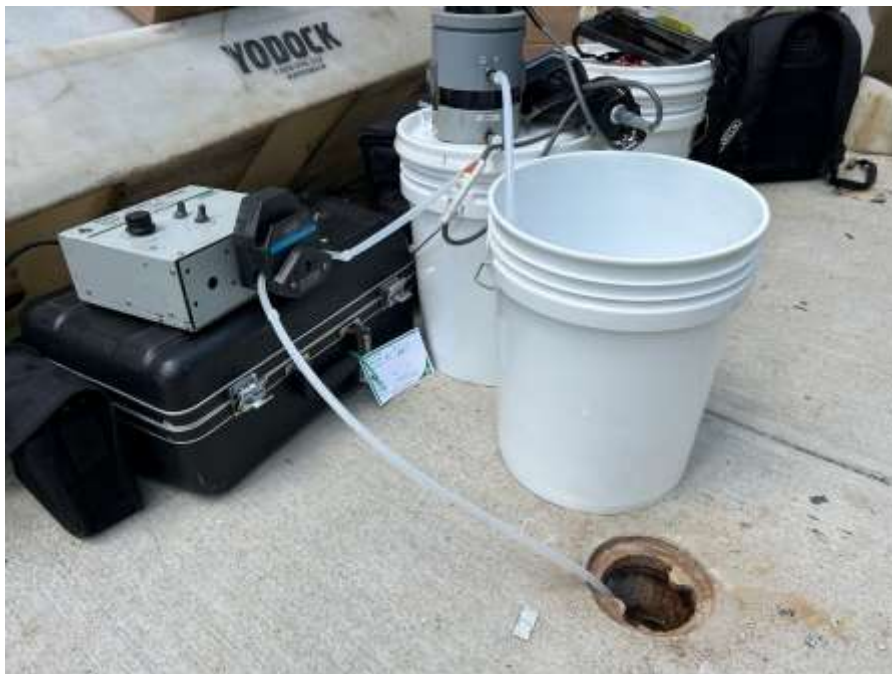
Photo 1: View of Langan purging monitoring well MW-2 along the Jackson Avenue sidewalk (facing southwest).
