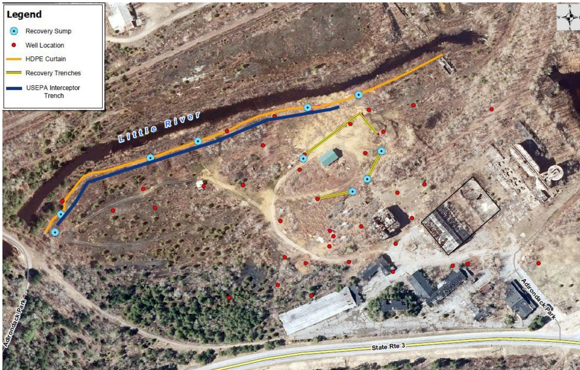
Figure 3 HDPE Curtain, Historic Recovery Trenches and Sumps, and USEPA Interceptor Trench
