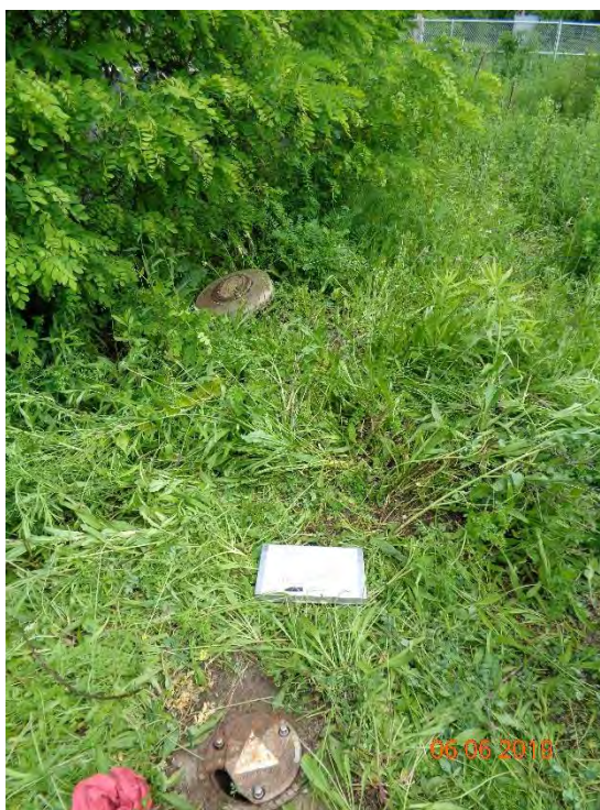
Photo 49 - View of PZ104S (foreground) and PZ104D (dislodged cover in background, could not locate well)
