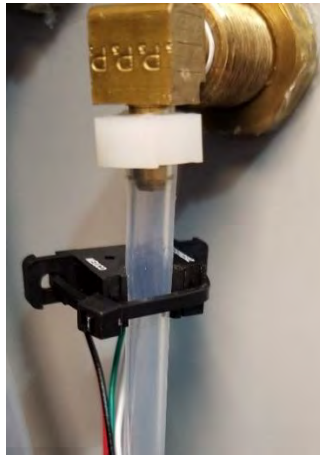
Figure 5-14: Optic sensor tubing installation
