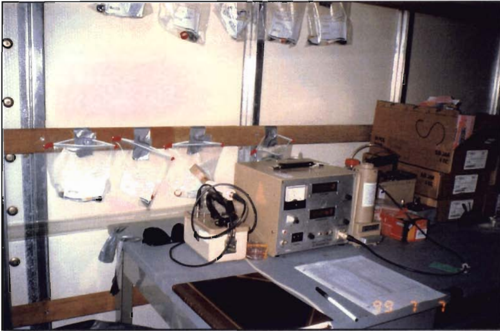
Trailer interior showing Model 2929 alpha/beta detector, film badge storage locations and other equipment.
