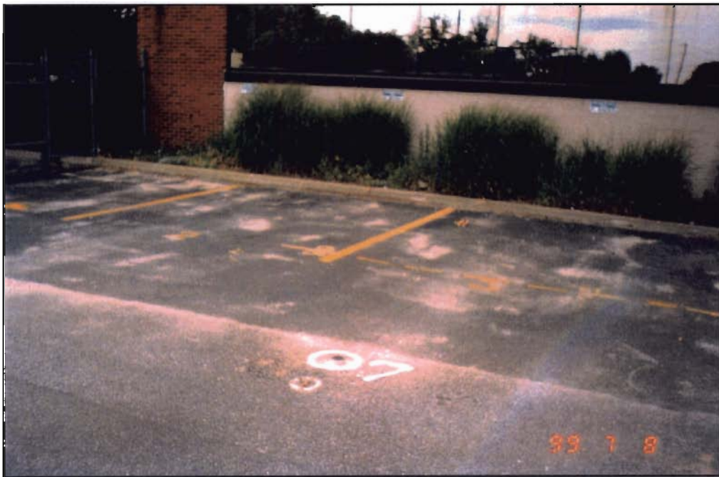
SB-007 was placed at Air Techniques, Inc. to evaluate subsurface conditions near the historic leaching pool.
