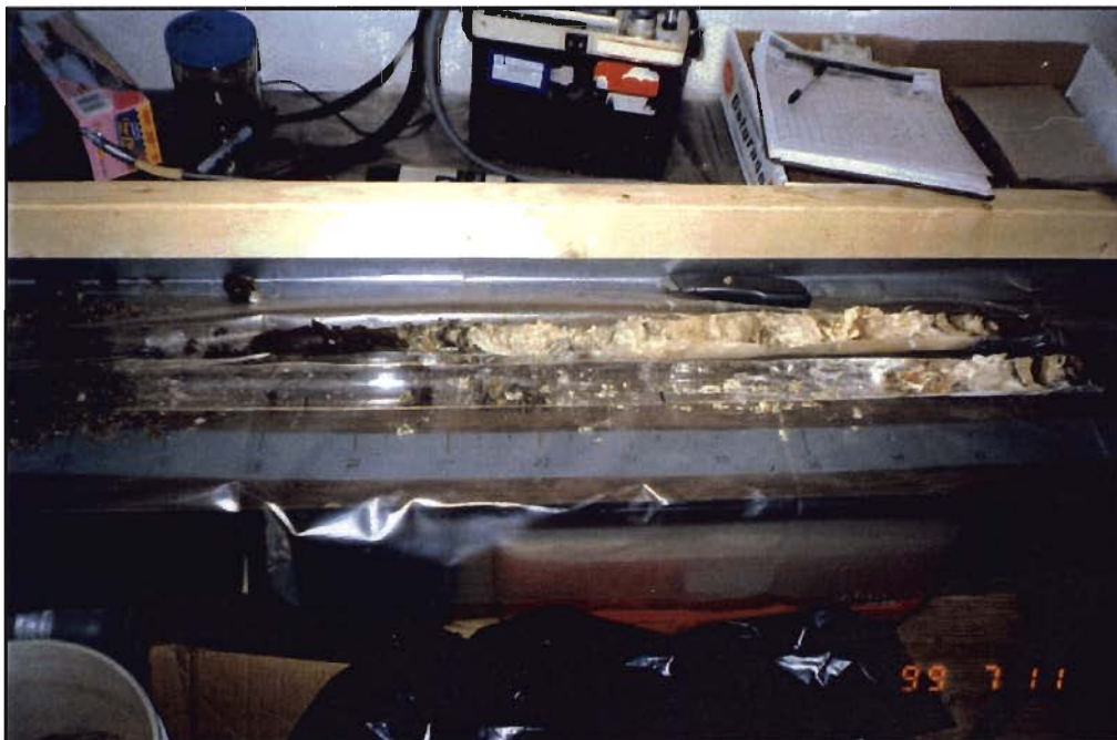
SB-024 contained pale yellow and green areas of significant above background readings of radiation.
