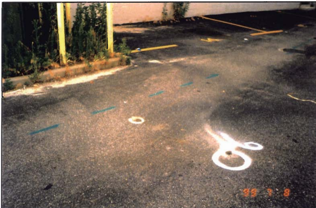
SB-006 was placed at Air Techniques, Inc. to evaluate subsurface conditions near the former leaching pool.
