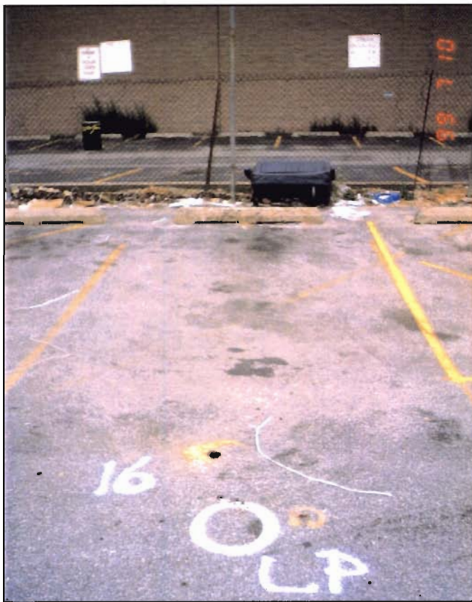
SB-016 was used to evaluate subsurface conditions adjacent to several historic underground structures (Magazine Distributors).
