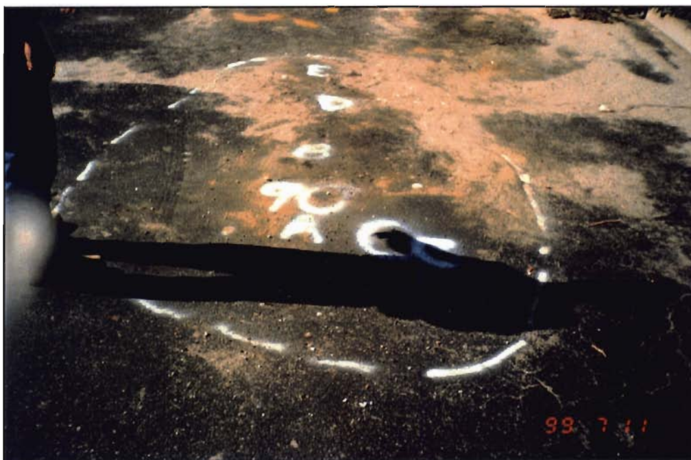
SB-009A - E were placed directly over an area of above background radiation readings found during the USRADs survey.
