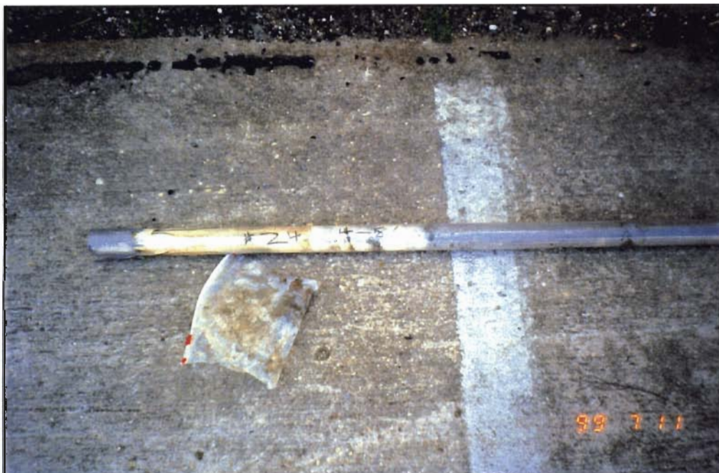
Sample soil core. This core from SB-024 (4-8 feet) exhibited layering indicative of a disposal area.
