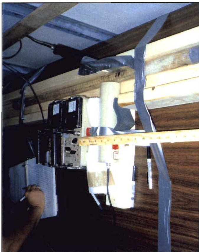
In field trailer radiation measurements were collected. (Note: pan-cake probe and 2" x 2" NaI probe)
